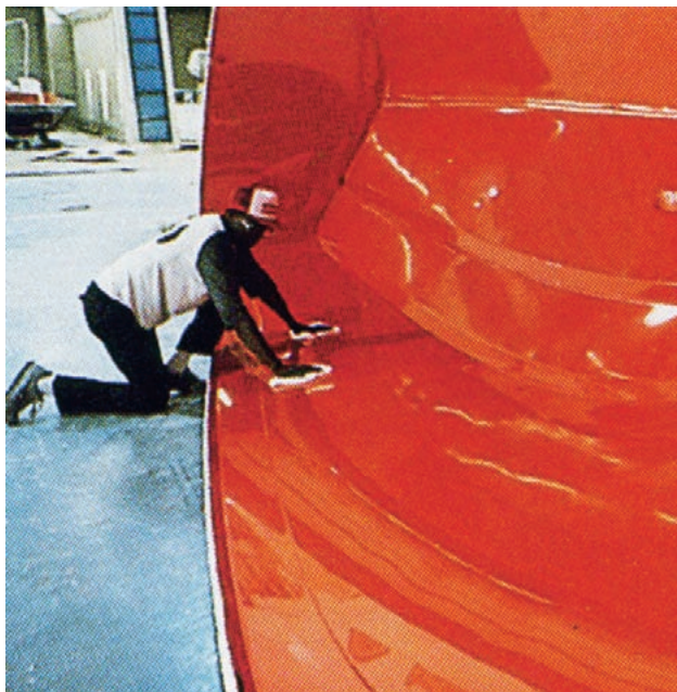
Polishing the hull molds in the new plant
