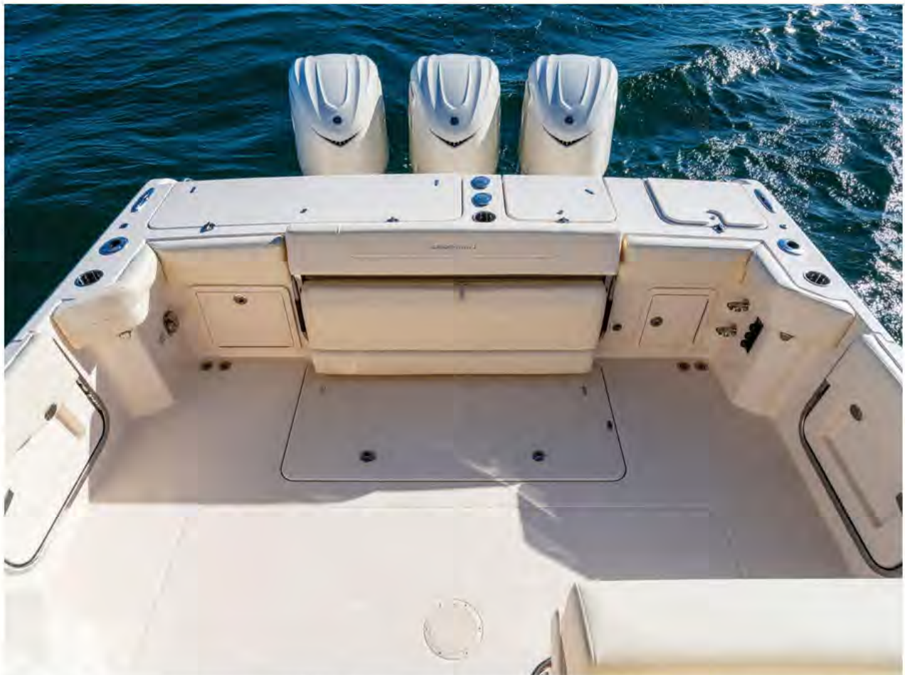
The 340's full transom incorporates a cooler, fishbox, livewell, fold-out bench seat, and gear and tackle storage. Courtesy Grady-White
