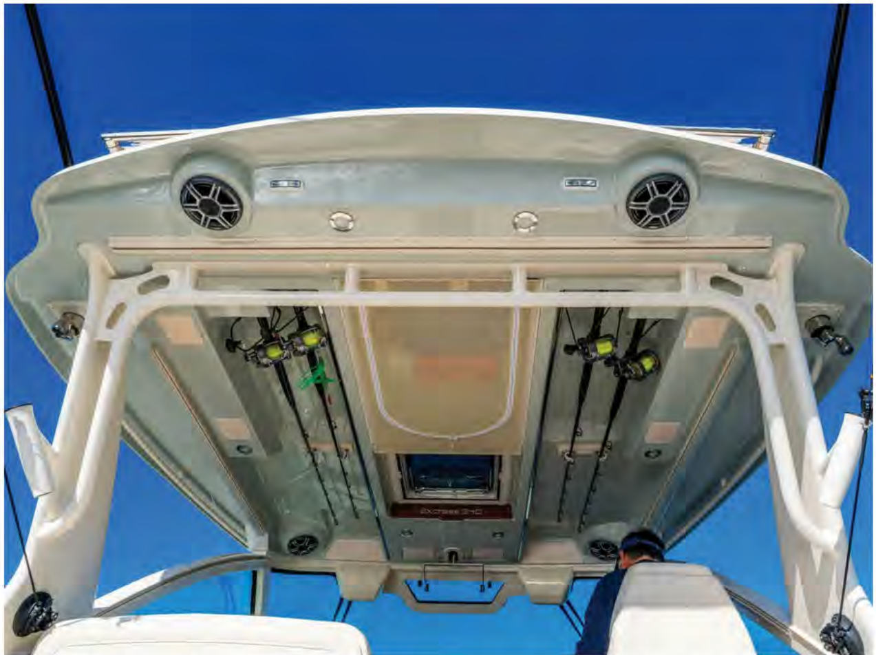
The Express 340 features a redesigned hardtop with overhead rod storage, indirect lighting, speaker pods and more. Courtesy Grady-White
